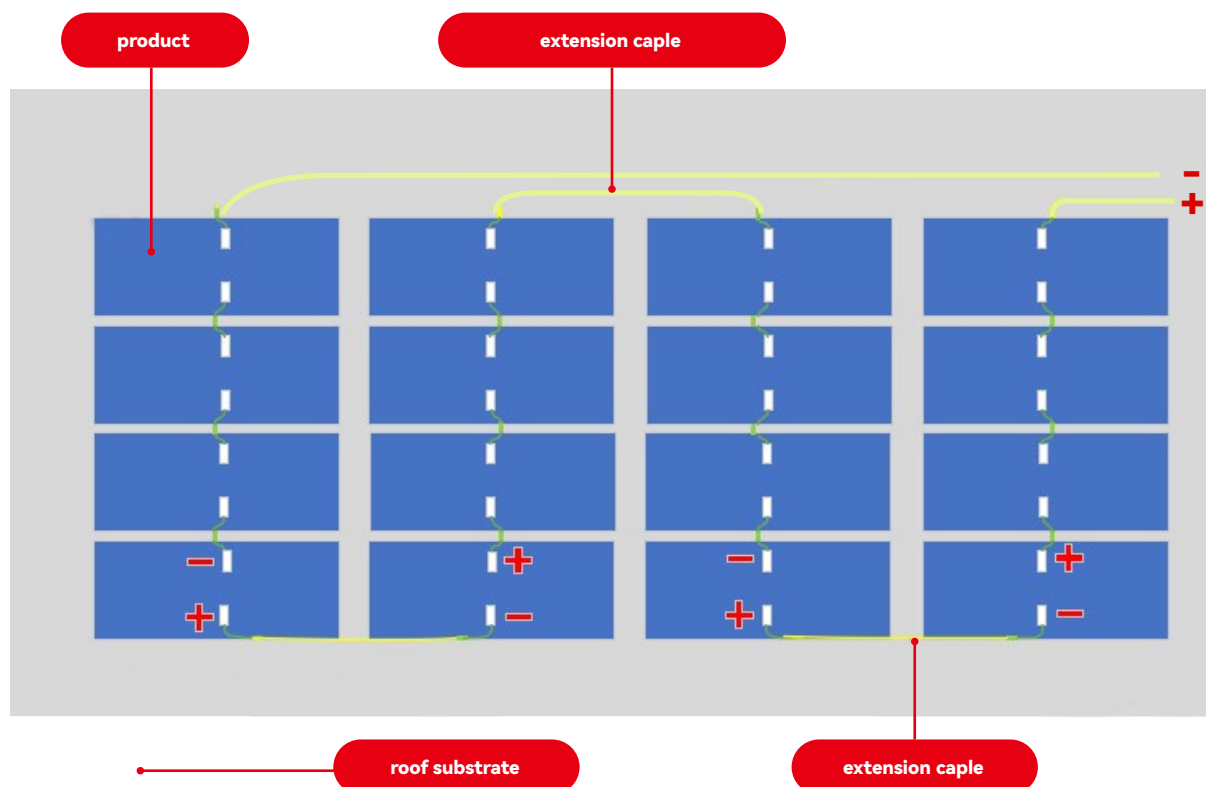
FIGURE 22 PRODUCT JUMPER CONNECTION OPERATION INSTRUCTIONS (FRONT VIEW)
