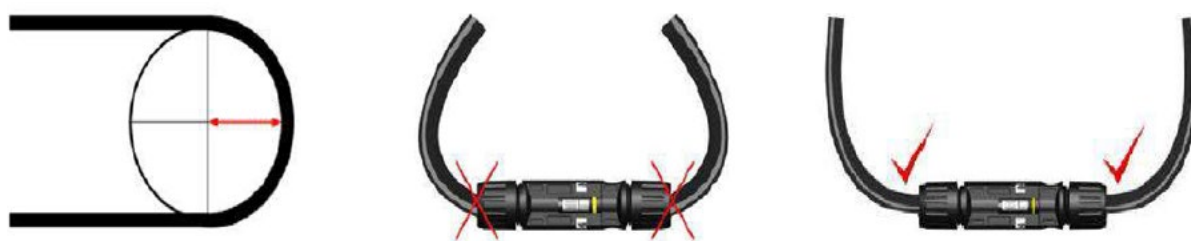
FIGURE 21 MINIMUM BENDING RADIUS OF THE CABLE
