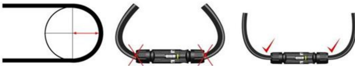
Figure 18 Minimum bending radius of the cable
