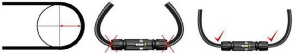
Figure: MINIMUM BENDING RADIUS OF THE CABLE
