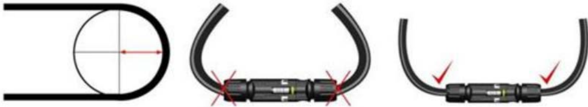
FIGURE 45 MINIMUM BENDING RADIUS OF THE CABLE
