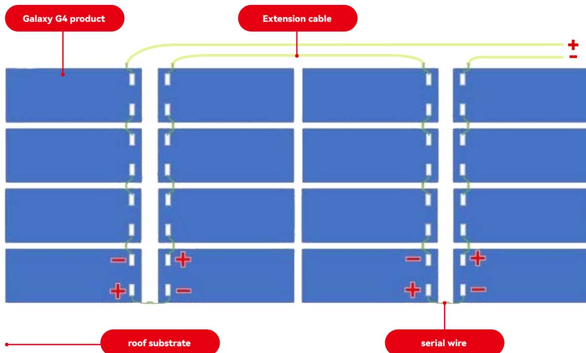
FIGURE 46 PRODUCT JUMPER CONNECTION OPERATION INSTRUCTIONS (FRONT VIEW)
